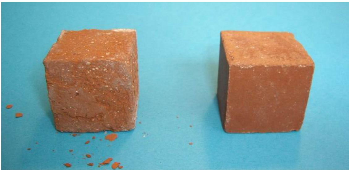
Laboratory brick models after 30 freezing-melting cycles: standard model and conserved sample
