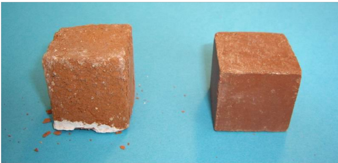
Laboratory brick models after a six-month long exposure to humidity: standard model and conserved sample
